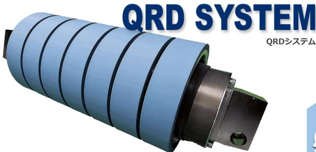
Automatic ink density control device. Individually divided ink ductor roller is operated by air cylinder and contact time with fountain roller is control by computer.
