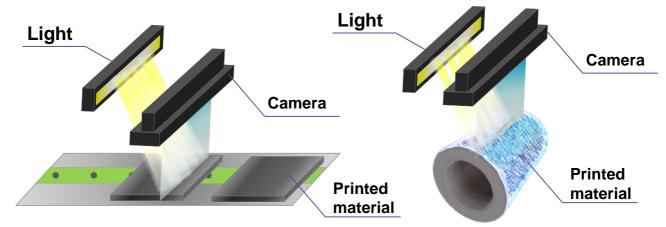
By simply capturing images of printed materials with a camera, the system compares the ink density at a specified position with the OK density already captured.
